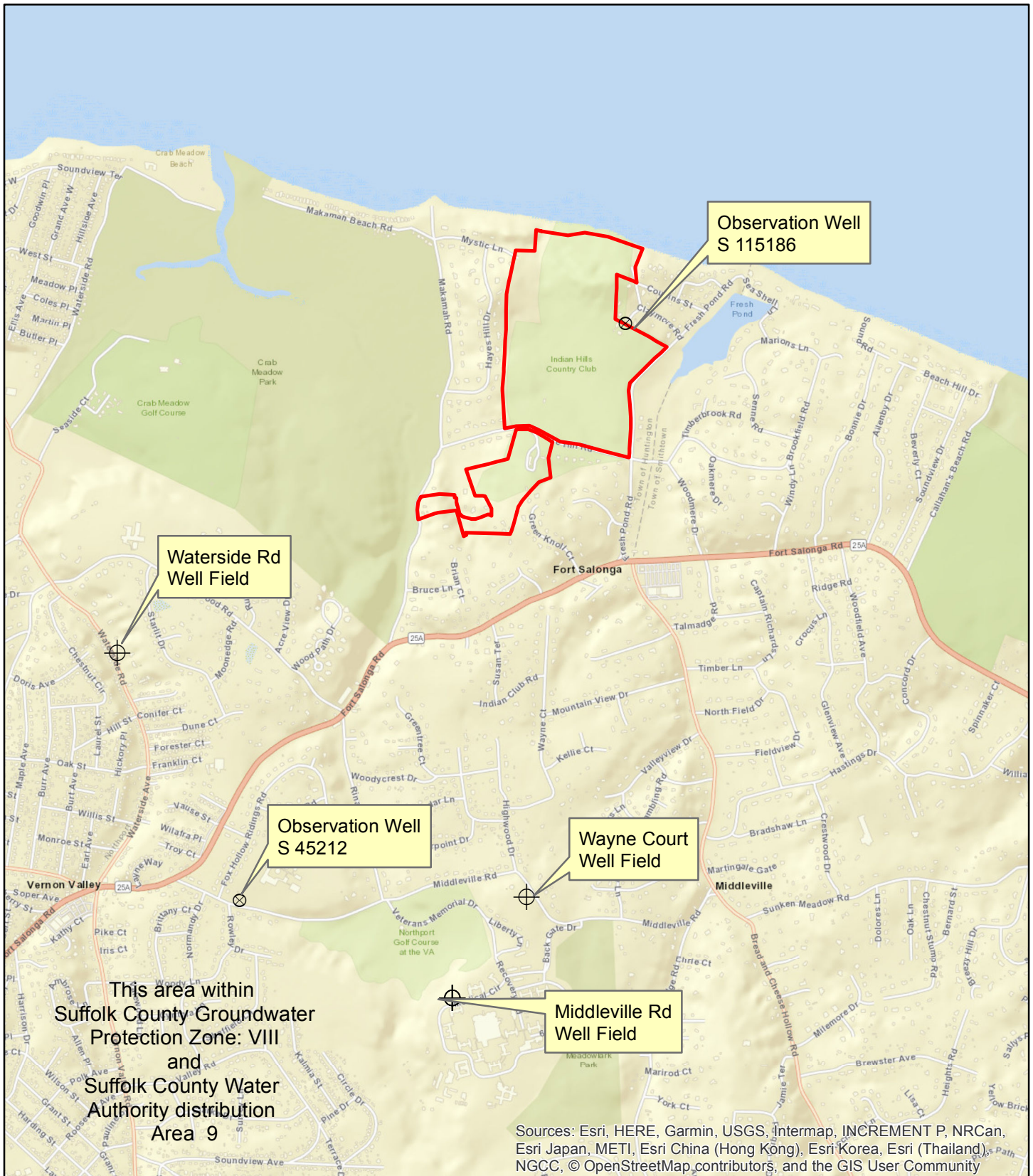
FIGURE 3-6 WATER SUPPLY AND MONITORING WELL MAP
